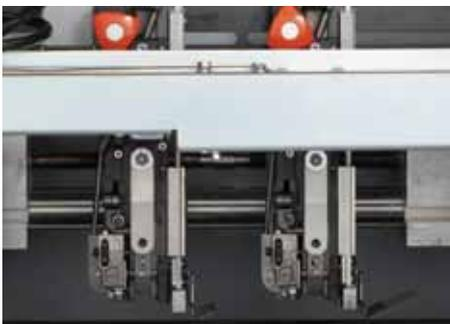
**The Hohner stitch heads automatically move into position when the job is recalled on the PC Controller. Optional 3-stitch and 4-stitch head kits are also available.**
