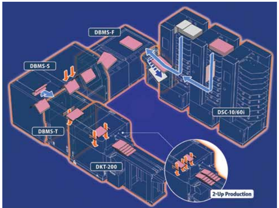
Saddle stitching at a glance: Take an inside look of the powerful and versatile DBMi as booklets are easily collated, scored, stitched, trimmed, and delivered.
