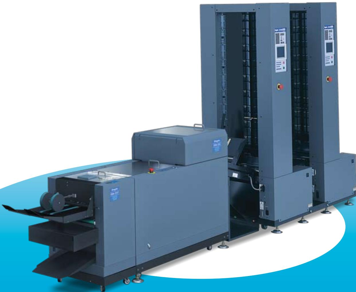
Duplo presents the first automatic finishing machine with an integrated spine press. The System 3500 is capable of producing up to 3,000 A5 booklets per hour and collating up to 9,000 A4 sets per hour whilst maintaining complete accuracy. The System 3500 comprises the versatile suction-fed 10/60 pro collator\* and the DBM-350/350T dynamic bookletmaker and trimmer.
